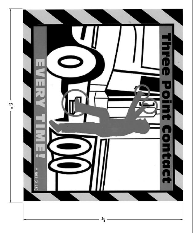
THERE SHALL BE A PERMANENT DECAL AFFIXED BY EACH ENTRY POINT. THE SAME PERMANENT DECAL SHALL BE AFFIXED BY EACH LADDER, PLATFORM OR STEP DESIGNED TO BE CLIMBED OR STEPPED ON. MEASUREMENTS OF DECAL ARE REFERENCED ABOVE.
